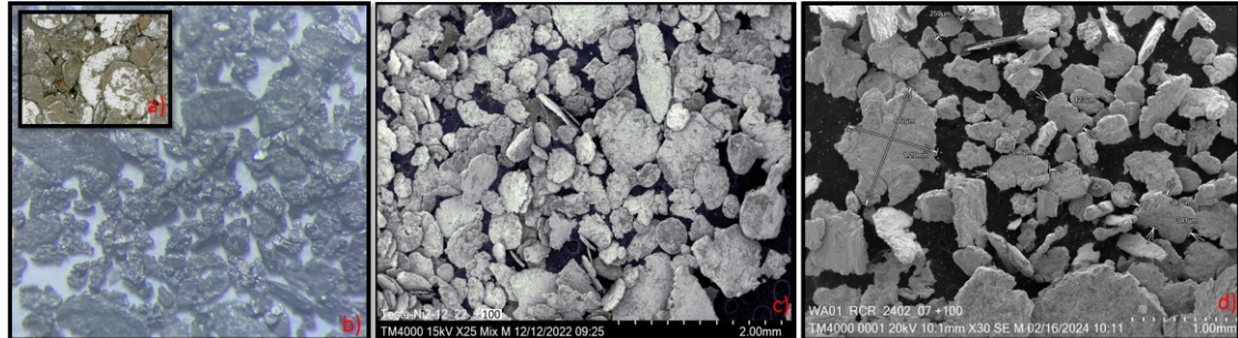
Figure 12. Left: a) Digital and b) optical microscope views. Coarse metallic iron agglomerates (150 \mu\text{m} size, with over 95% Fe Grade), Middle: c) and Right: d) SEM morphology analysis after reduction (150 \mu\text{m} ).
