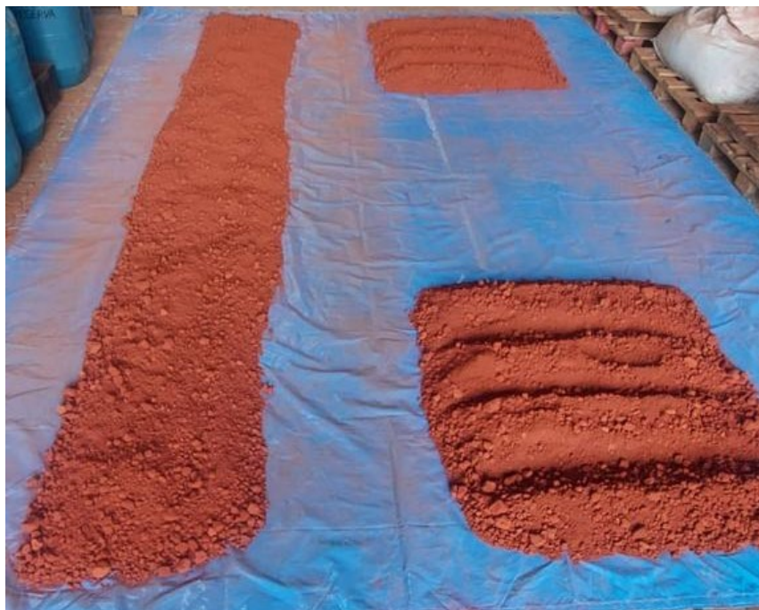
Figure 5. Representative sample received from Hydro Alunorte, homogenized, and quartered for characterization and tests.
