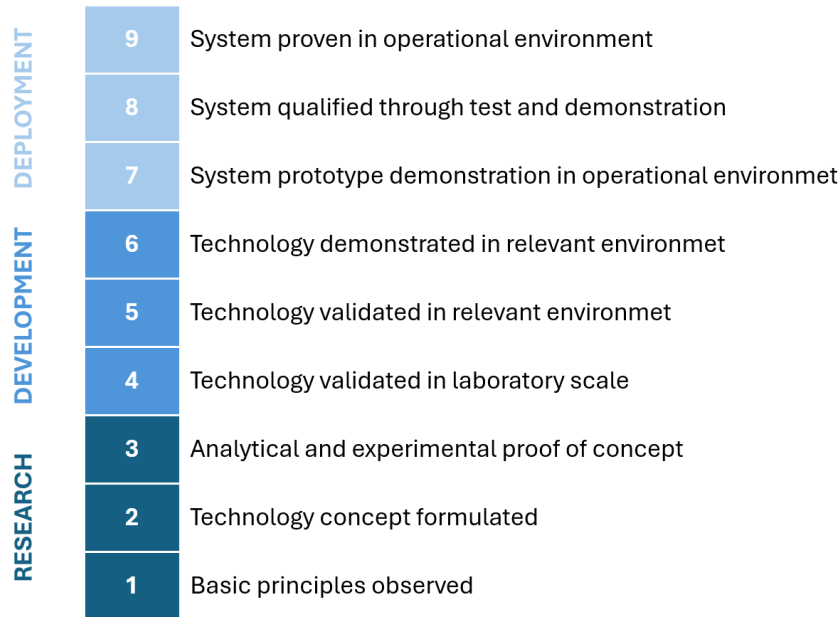
Figure 4. Technology Readiness Level (TRL) methodology for the validation of new technologies [19].
